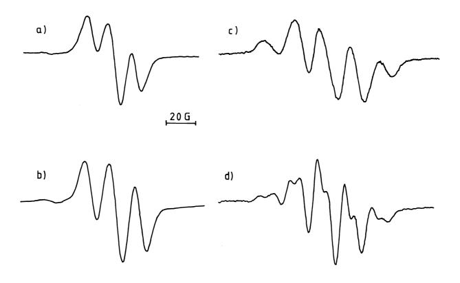
Fig. 1. ESR spectra of (a)  $1^{\frac{1}{2}}$  at 123 K; (b)  $2^{\frac{1}{2}}$  at 107 K; (c)  $3^{\frac{1}{2}}$  at 133 K; (d)  $4^{\frac{1}{2}}$  at 133 K in frozen CFCl<sub>3</sub>.
